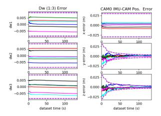
Fig. 5. Evaluation on  $tum\_room$  with one-axis rotation using  $imu22\{D_{w6}, D_{a6}, {}^I_a \mathbf{R}, \mathbf{T}_{g9}\}$ . Note that the estimation errors and  $3\sigma$  bounds for  $d_{w1}, d_{w2}, d_{w3}$ , and the IMU-camera position calibration along the rotation axis cannot converge.
