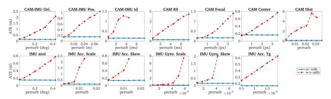
Fig. 4. Average absolute trajectory errors (ATE) over five runs using  $imu22\{\mathbf{D}_{w6}, \mathbf{D}_{a6}, {}^{I}_{a}\mathbf{R}, \mathbf{T}_{g9}\}$  and radtan on the  $tum\_corridor$  with full 3-D motion given different levels of perturbation. Only the calibrated parameter was perturbed while other parameters were initialized to their true values and not estimated. ATE above eight meters were not reported and can be considered as divergence.
