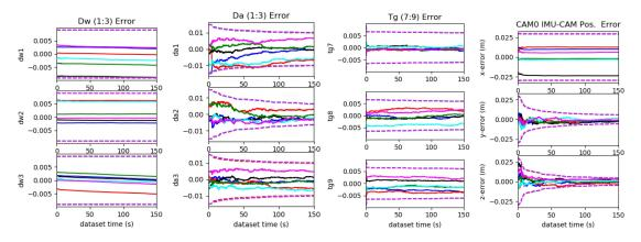
Fig. 7. Evaluation on  $udel\_gore$  with planar motion using  $imu22\{\mathbf{D}_{w6}, \mathbf{D}_{a6}, \frac{I}{a}\mathbf{R}, \mathbf{T}_{g9}\}$  and radtan. With planar motion, the estimation errors, and  $3\sigma$  bounds of  $d_{w1}, d_{w2}, d_{w3}, t_{g7}, t_{g8}, t_{g9}$ , and the IMU-camera position cannot converge. Due to the lack of motion excitation, the parameters of  $\mathbf{D}_a$  and  $\frac{I}{a}\mathbf{R}$  converge much slower than the other motion cases.
