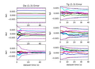
Fig. 6. Evaluation on the  $sine\_3$  d with constant acceleration along x-axis using  $imu22\{\mathbf{D}_{m6}, \mathbf{D}_{a6}, {}^I_a\mathbf{R}, \mathbf{T}_{g9}\}$ . The estimation errors and  $3\sigma$  bounds for  $d_{a1}$ , pitch and yaw of  ${}^I_a\mathbf{R}$  cannot converge. Note that  $t_{g1}$ ,  $t_{g2}$ , and  $t_{g3}$  also converge very slow.
