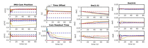
Fig. 16. Calibration results (four VI-Rig planar motion datasets with colored solid lines) for  ${}^{C}\mathbf{p}_{I}$ ,  $t_{d}$ ,  $t_{r}$ , and  $\mathbf{D}_{w}$  of the proposed system evaluated using imu2{ $\mathbf{D}_{w6}$ ,  $\mathbf{D}_{a6}$ ,  ${}^{I}_{a}\mathbf{R}$ } and equi-dist. Red and blue dotted lines denote the reference value from Kalibr and initial (perturbed) values, respectively. The y component of  ${}^{C}\mathbf{p}_{I}$ ,  $dw_{1}$ ,  $dw_{2}$ , and  $dw_{3}$  diverges.
