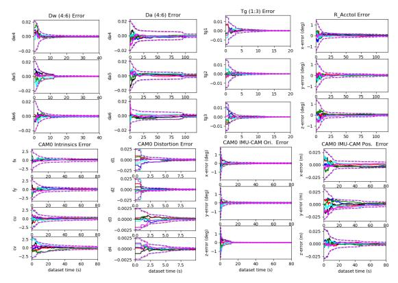
Fig. 3. Evaluation on  $tum\_corridor$  with fully excited motion (using  $imu22\{\mathbf{D}_{w6},\mathbf{D}_{a6},\frac{I}{a}\mathbf{R},\mathbf{T}_{g9}\}$  and radtan).  $3\sigma$  bounds (dotted lines) and estimation errors (solid lines) for six different runs (different colors) are shown.
