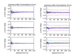
Fig. 8. Camera to IMU orientation errors when using IMU imu2  $\{\mathbf{D}_{w6}, \mathbf{D}_{a6}, \mathbf{D}_{a6}, \mathbf{I}_{a}\mathbf{R}\}$  (left) and the over parameterized imu5  $\{\mathbf{D}_{w6}, \mathbf{D}_{a6}, \frac{I}{w}\mathbf{R}, \frac{I}{a}\mathbf{R}\}$  (right). Note that only the IMU intrinsics and relative pose between IMU and camera were calibrated online.
