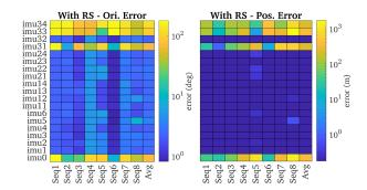
Fig. 11. Results on TUM RS VIO dataset *with* readout time calibration, with different IMU intrinsic models. The averaged ATE of five runs in degree (top) and meters (bottom) are provided. Note that camera intrinsics, and IMU-camera spatial-temporal parameters are calibrated.
