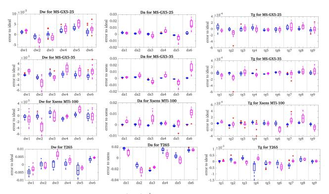
Fig. 14. Comparison of the proposed method with  $imu6\{D'_{w6}, D'_{a6}, {}^I_w\mathbf{R}, \mathbf{T}_{g9}\}$  and Kalibr relative to the "ideal" sensor intrinsics. Kalibr (magenta, right in each group) was run with all cameras and IMUs available over ten datasets, while the proposed system (blue, left) was run with either the Blackfly camera or left T265 fisheye resulting in 20 runs. Red + denotes outliers.
