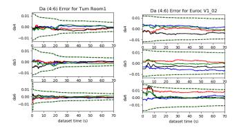
Fig. 15. Evaluation of the proposed system for  $\mathbf{D}_a$  with  $tum\_rooml$  (left) and  $EuRoc\ VI\_02$  (right) trajectories using  $imu2\{\mathbf{D}_{w6},\ \mathbf{D}_{a6},\ \overline{{}}_a^I\mathbf{R}\}$ .  $3\sigma$  (dotted lines) and estimation errors (solid lines) for four different runs (different colors) are drawn. The convergence of  $d_{a4}$ ,  $d_{a5}$  and  $d_{a6}$  is poor for the  $EuRoc\ VI\_02$  due to lack of motion excitation.
