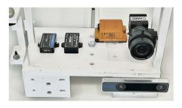
Fig. 12. Visual-Inertial Sensor Rig contains a MS-GX5-25 IMU, MS-GX5-35, Xsens MTi 100, FLIR Blackfly camera, and RealSense T265 tracking camera (containing an integrated IMU and a fisheye stereo camera).
