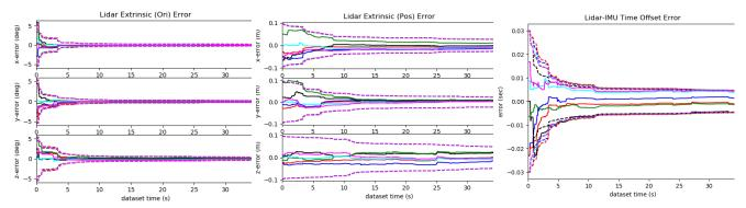
Fig. 5: Calibration errors of each parameter (solid) and  $3\sigma$  bound (dotted) for six different runs under random motion. Each colors denote runs with different realization of the measurement noise and the initial values. Both the estimation errors and  $3\sigma$  bounds can converge in about 10 seconds.
