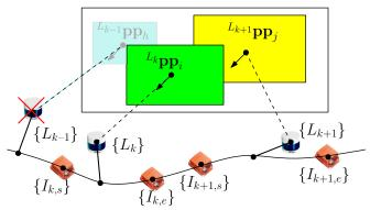
Fig. 3: Selection of LiDAR measurements for the update.  $\{I\}$  and  $\{L\}$  indicate the historical IMU poses and LiDAR frames at measurement time, respectively. In this example, the LiDAR measurement at  $t_k$  and  $t_{k+1}$  are collected for the update, while at  $t_{k-1}$  is not because the IMU poses cannot bound the measurement.
