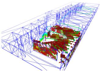
Fig. 1: The proposed *MINS* working in simulations. The green represent the plane patches extracted from the LiDAR point cloud, the red are the merged plane patches, and the yellow are the patches used to update the estimator. Green and light blue paths are the estimated and ground truth trajectories, respectively.
