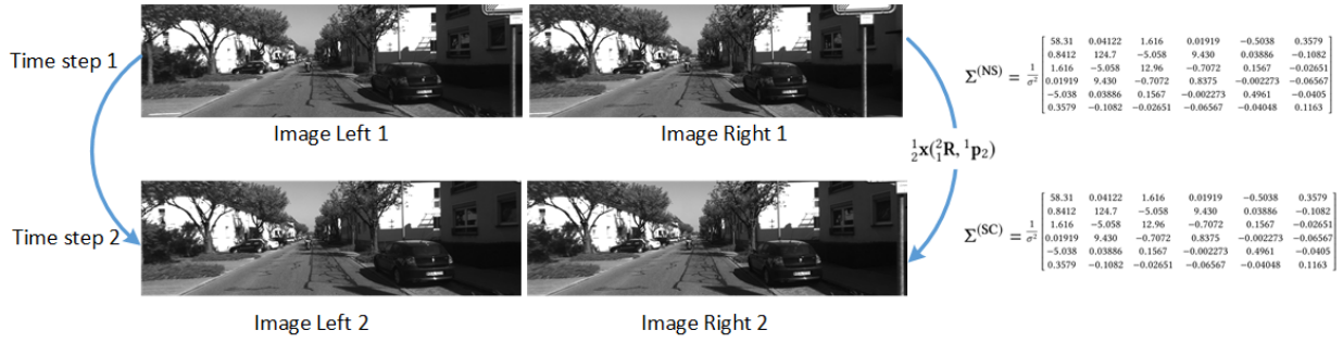
Fig. 2. A typical vision factor for visual odometry. \frac{1}{2}\mathbf{x}_1^T \mathbf{R}_1 \mathbf{p}_2 represents the transformation from stereo camera pose 1 to pose 2, where \mathbf{R}_1 and \mathbf{p}_2 denote the rotation and translation between pose 1 and pose 2, respectively.
